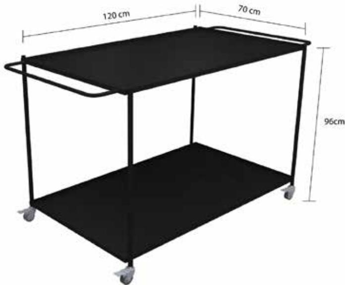
Figure 10: The Measurements of the Proposed Industrial Ergonomic Trolley-Lifter
