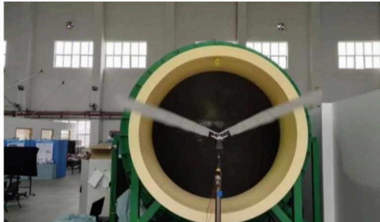
Fig. 6 Ground test bench for flapping mechanism [28]
