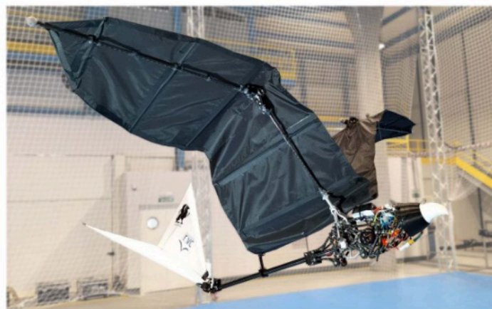
Fig. 7 Flapping wing robot equipped with an elastic wing [2]
