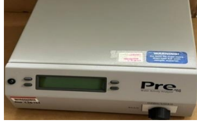
Figure 3.12: Water activity meter (FA-st Lab, GBX, France)
