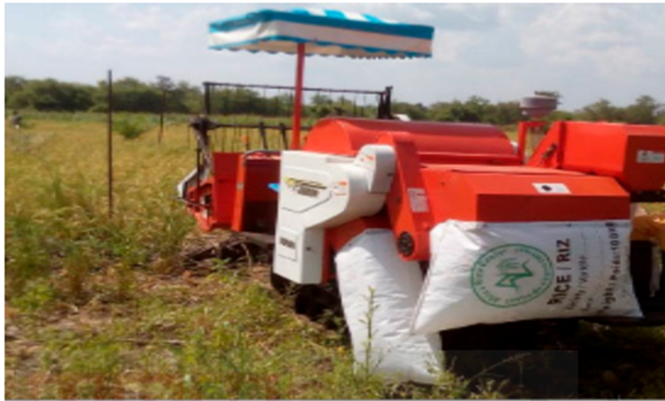
Figure 2.12: Grain loss collection in a woven sack from the concave and rear of the combine harvester (Amponsah et al., 2017)
