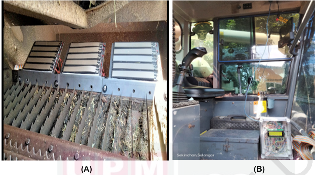
Figure 3.31: Illustration of the grain loss monitoring system installation (A-Installed grain loss sensitive plates, B-Monitoring circuit box at operators' cabin)
