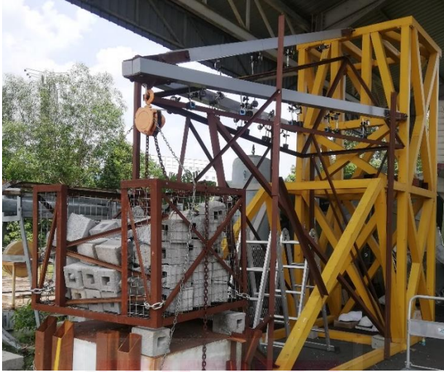
Figure 3.15: Assemble cross-arm layout during creep test.
