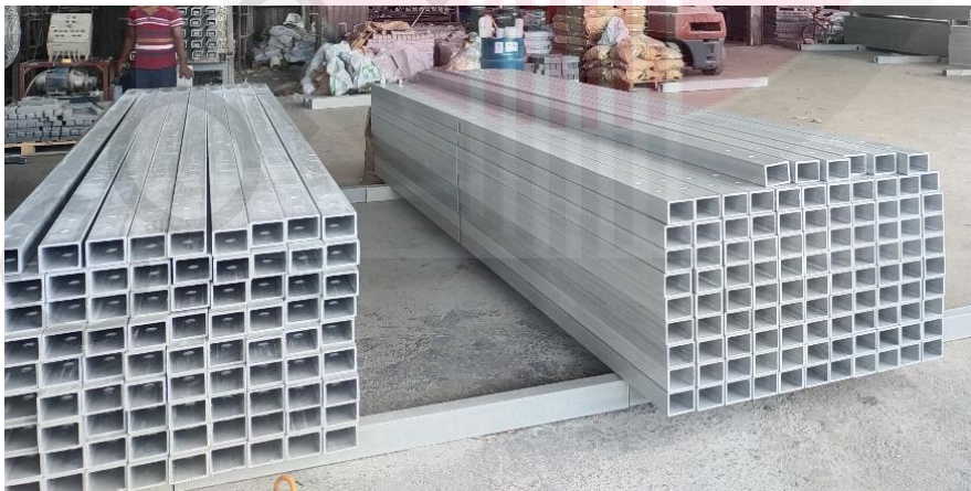
Figure 3.2: Complete mass manufactured PGFRPC cross-arm.
