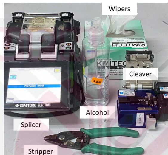
Figure 3.3: Equipment for SMTF fabrication.
