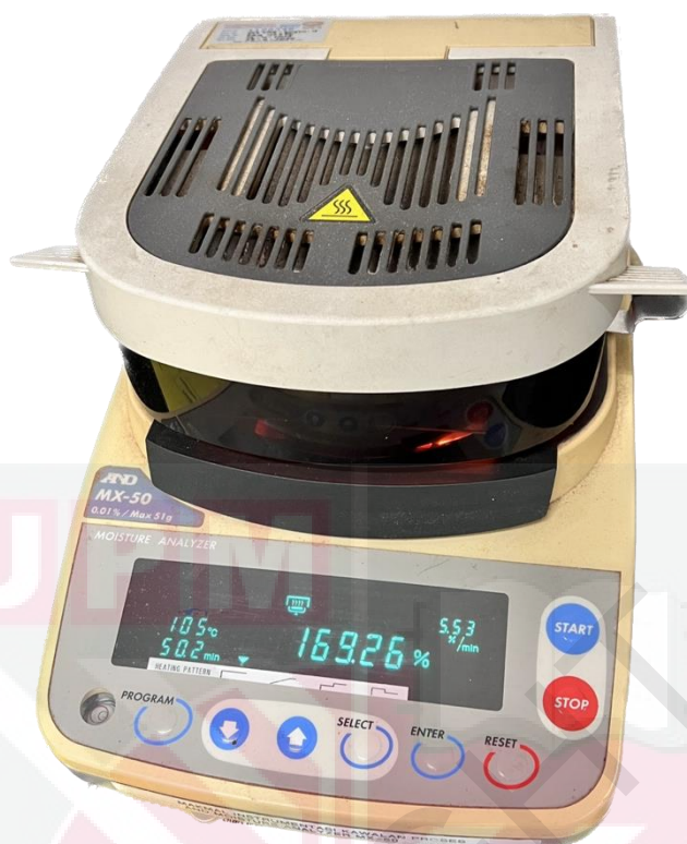
Figure 3.10: Moisture analyzer used for determining the percentage of moisture content in Parkia speciosa Hassk powder
