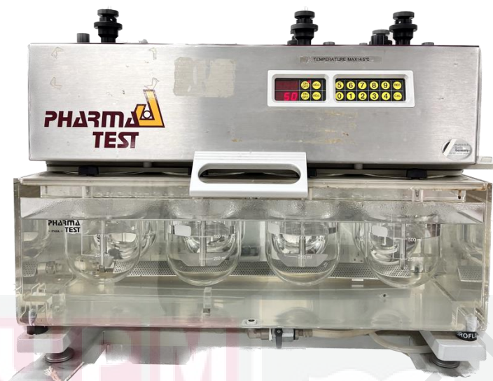
Figure 3.13: Dissolution tester used to measure the dissolution time
