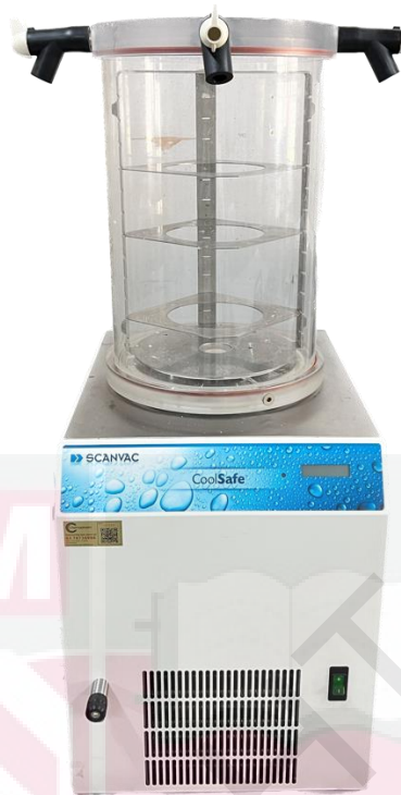
Figure 3.4: ScanVac freeze dryer used for freeze-drying the Parkia speciosa Hassk seeds
