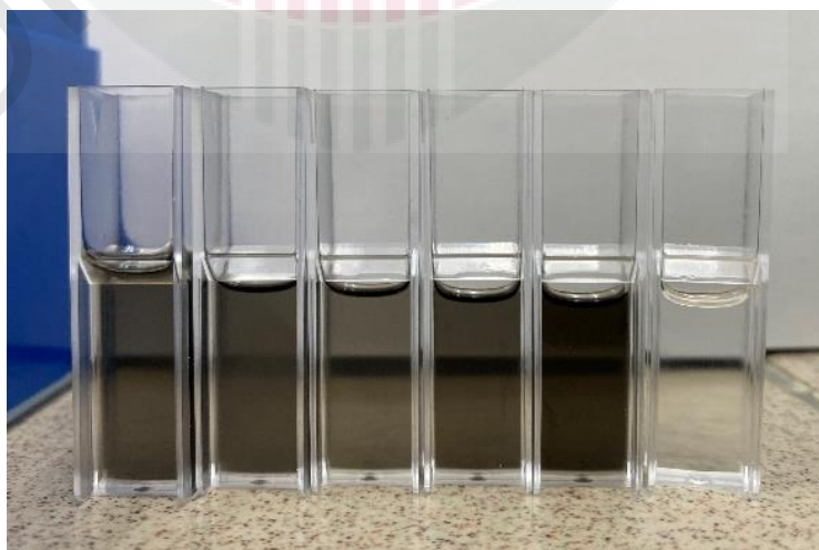
Figure 4.3 : The MWCNT samples on cuvette for UV-vis testing
