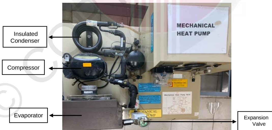
Figure 3.7 : Top view of mechanical heat pump R514
