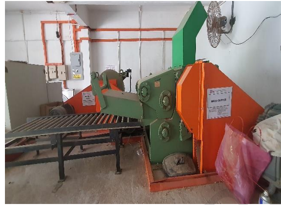
A.8 Crusher machine
