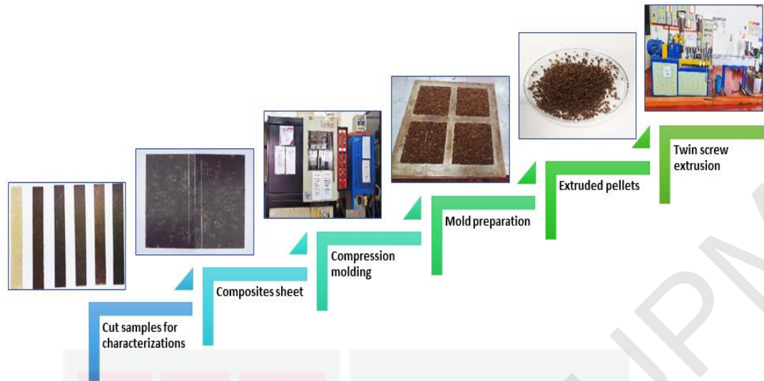
Figure 3.4 : Fabrication Process of BF-KF/PLA Hybrid Composites
