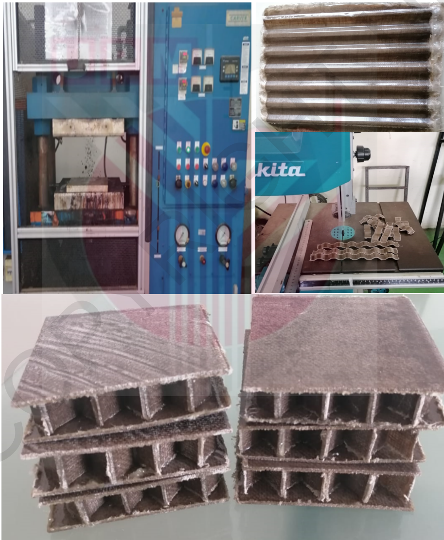
Figure 3.12: Photos of the complete process of fabrication of honeycomb core sandwich structure
