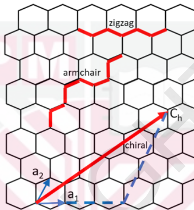
Figure 2.1: Schematic of how graphene can be rolled into various chirality of CNT
