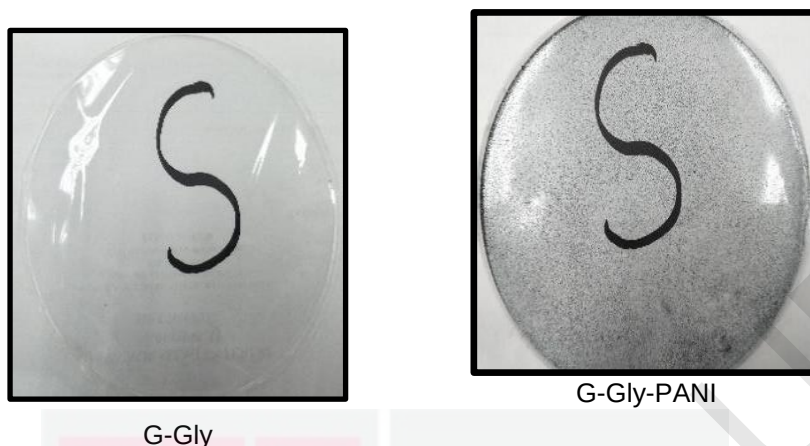
Figure 4.13: Digital photograph of developed active gelatin-based film; Left: G-Gly and Right: G-Gly-PANI
