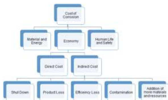
Figure 1. Cost incurred due to corrosion [5]
