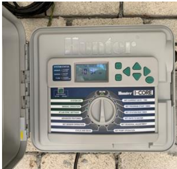
Figure D.13: Hunter iCORE used as a centre of the system
