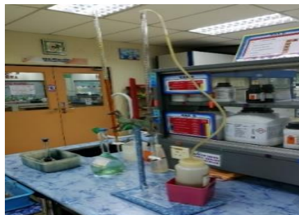
Figure A.8: Titration process setup
