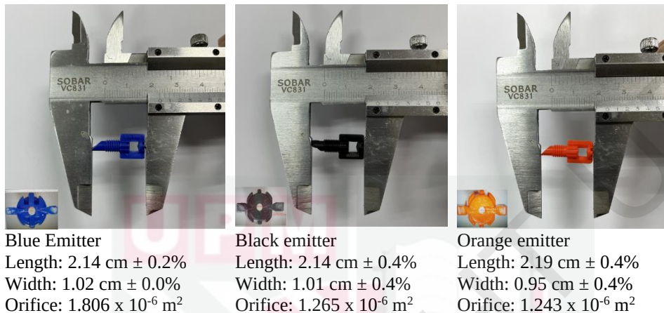
Figure 4.28: Specification of a low-cost emitter according to colour code
