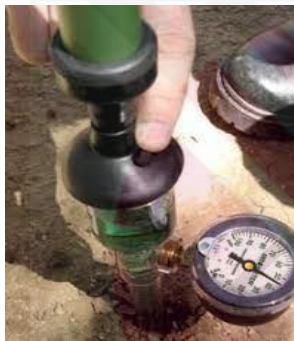
Figure D.18: Air bleed was used to release air compression inside the tensiometer
