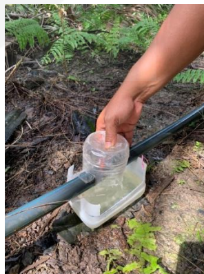
Figure E.10: Custom plastic protective case for water measurement
