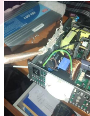
Figure 4.54: Inverter circuit board burns because of lizard
