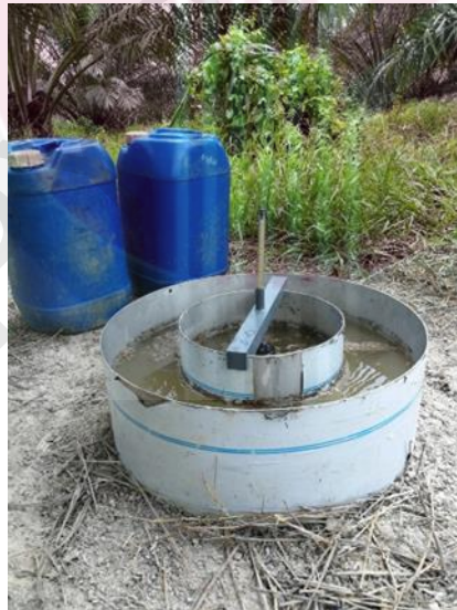
Figure 3.17: Double-ring infiltrometer setup for each location
