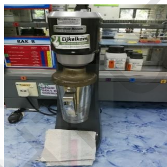
Figure A.2: Apparatus used to stir the solution
