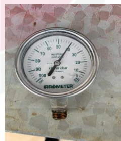
Figure 4.52: Tensiometer gauge needle stuck at a higher value
