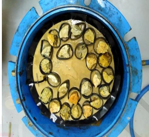
Figure 3.6: The arrangement of the sample in the pressure chamber
