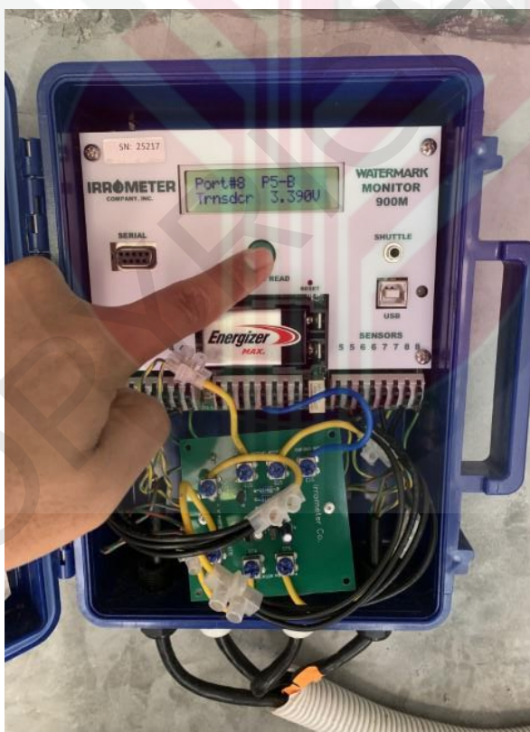
Figure D.22: LCD display shows the value of the data
