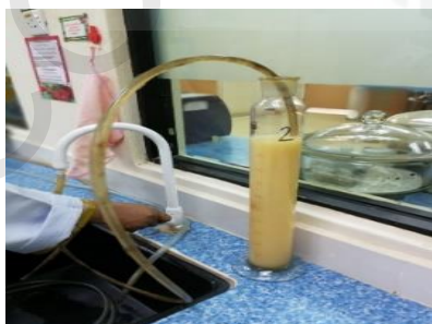
Figure A.5: Water was added to the supernatant until the colour of the solution became clear
