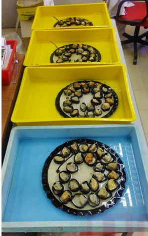
Figure 3.5: Saturation process before sample transfer into the pressure chamber
