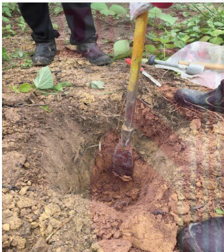
Figure 3.13: Soil was dug by using a chisel to open enough space for sampling purposes
