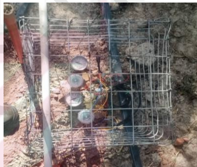
Figure D.19: Special cage used to protect tensiometer
