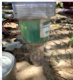
Figure 4.51: Water remains at the reservoir due to the overtightening lid
