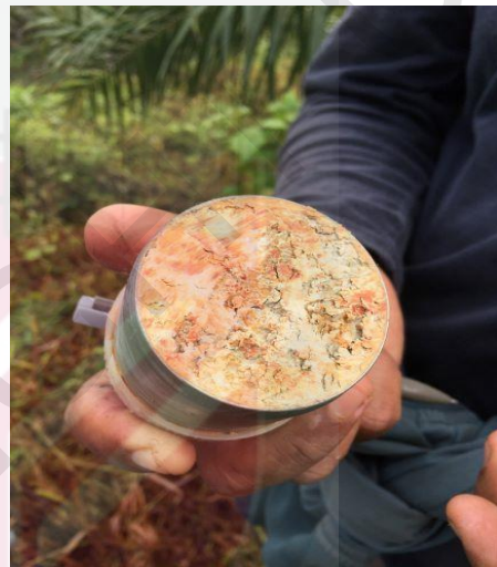
Figure 3.14: Sample in the ring that will be enclosed with the lid to send to the laboratory
