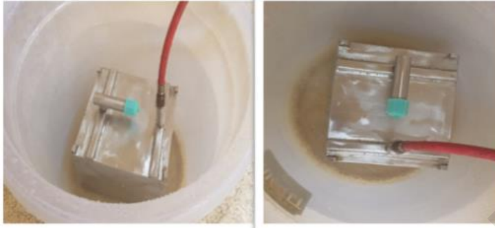
Figure 3.22: Leak detection using water
