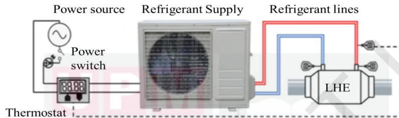
Figure A14: The Vehicle air-conditioning simulator circuit connection and parts
