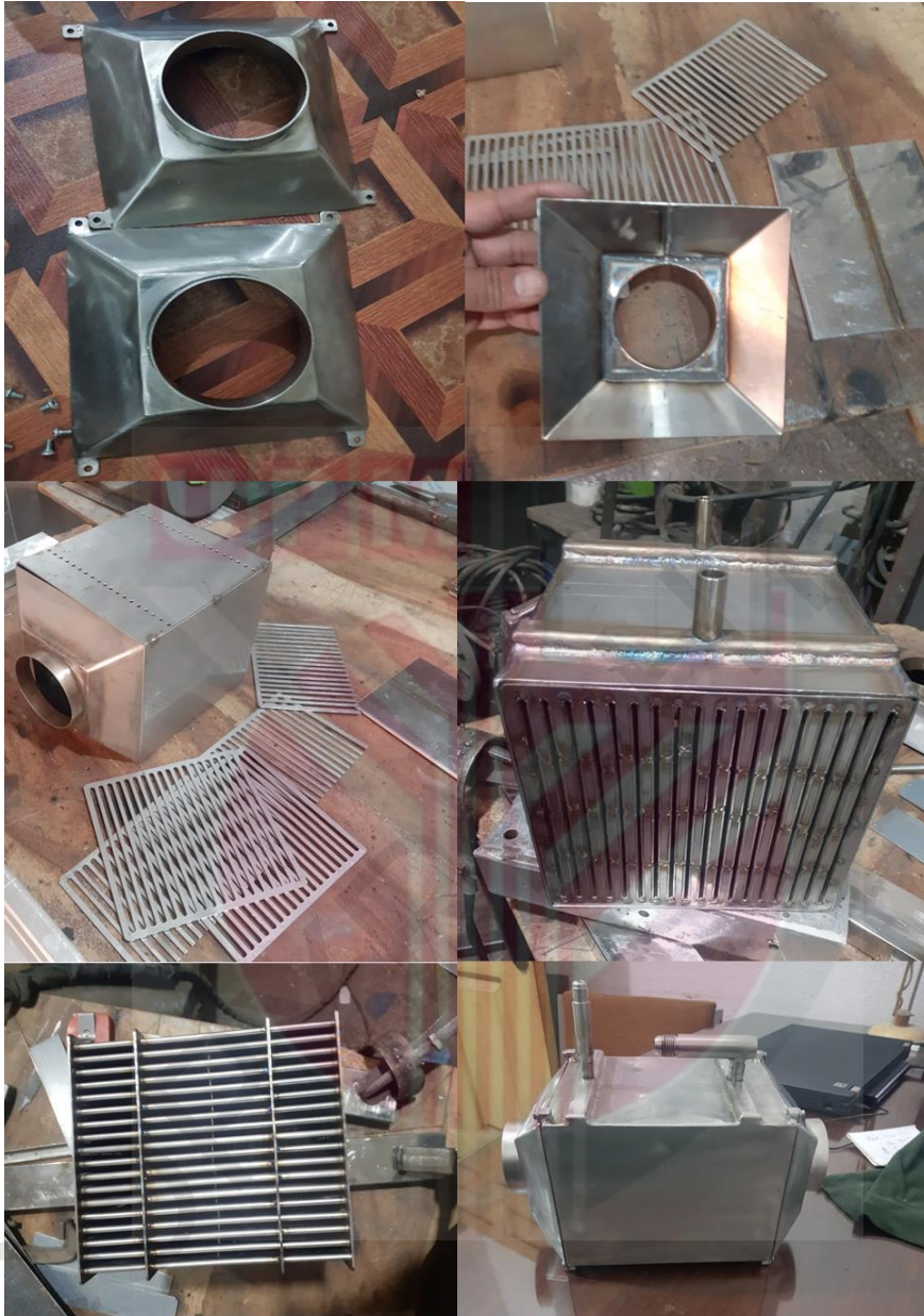
Figure A9: Fabrication of LHE (continued)
