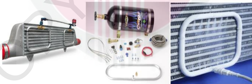
Figure 2.8: Intercooler sprayer system (Choo, 2005)
