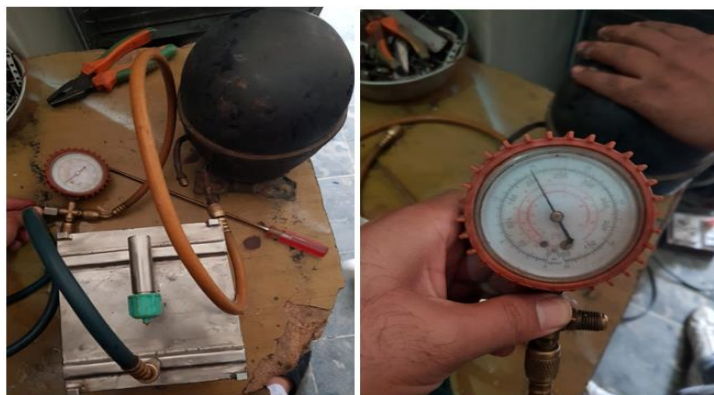
Figure 3.20: Pressure drop test method using a compressor
