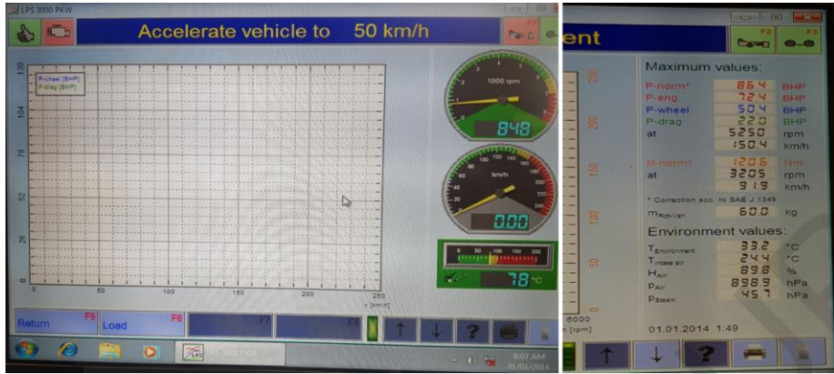
Figure A20: MAHA Chassis dynamometer discrete power result illustrating test results
