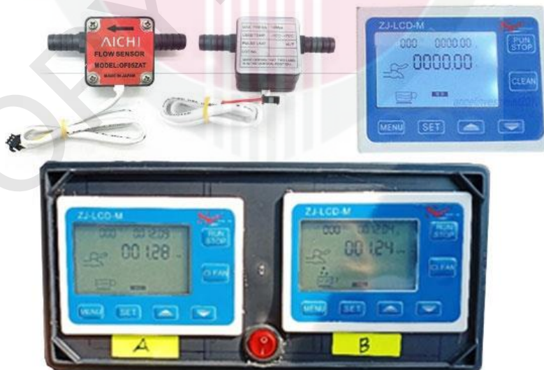
Figure 3.36: Fuel meters and measurement devices used to measure the fuel consumption
