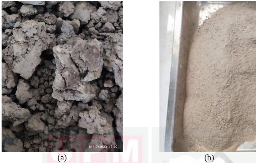
Figure 3.3: Samples (a) before and (b) after grinding process using soil grinder
