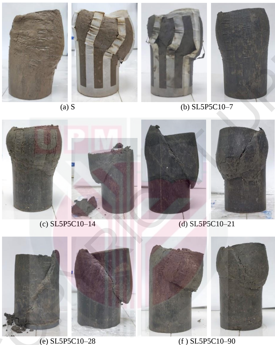
Figure 4.14: Triaxial specimens after failure for SL5P5C10 specimens on various curing durations compared to (a) control specimen, (b) 7, (c) 14, (d) 21, (e) 28, and (f) 90 curing days
