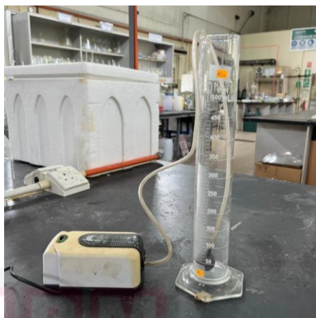
Figure 3.13: The aeration-based foaming tendency assay
