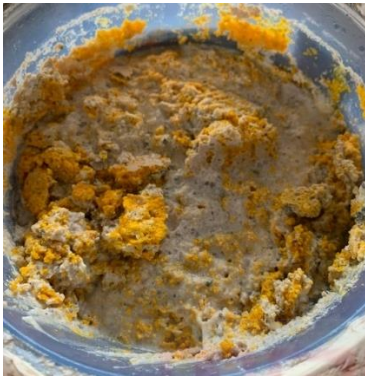
Figure 4.53: Scum formation in Tank 1 two-stage AD treated with palm oil
