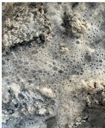
Figure 4.71: Foam formation in tank 1 for blank
