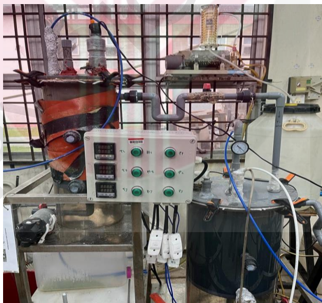
Figure 3.11: Experimental set-up of two-stage anaerobic digester
