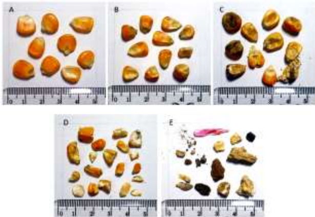
Fig. 2: Physical corn kernel pictures, A=normal; B=damage kernels; C=moldy kernels; D=broken kernels; and E=foreign materials.
