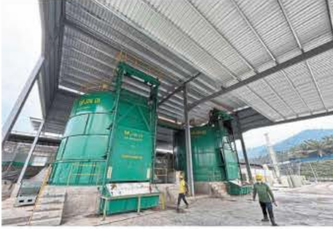
Two 200 cubic metre towers where fresh manure is composted (above) and a trench system, still under construction (right), are part of the waste management systems at QL Poultry Farms in Pajam.
