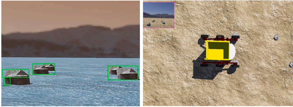
Fig. 6. Webots world scene showing the six-wheel robot navigating uneven turf with randomized stone obstacles.
