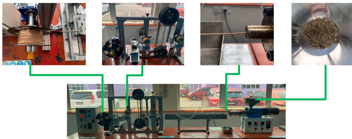
Fig. 2. Filament fabrication process of rPLA-PDA/KF.
