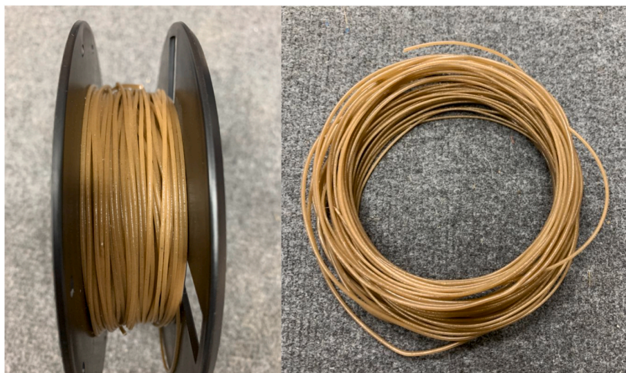
Fig. 3. Sample of 3D Printing filament rPLA-PDA/KF5 (5 wt%) for 1.75 mm average diameter.
