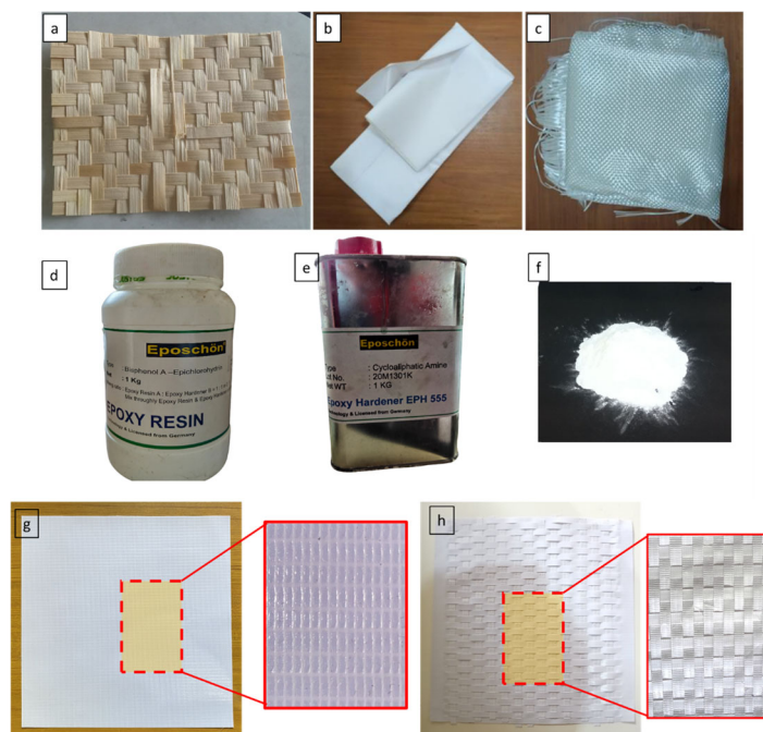
Figure 1. Materials used in this study: (a) Bamboo, (b) Flex banner, (c) Glass Fiber, (d) Epoxy, (e) Hardener, (f) CaCO 3 filler, (g) Flex banner before weaving, (h) Flex banner after weaving.
