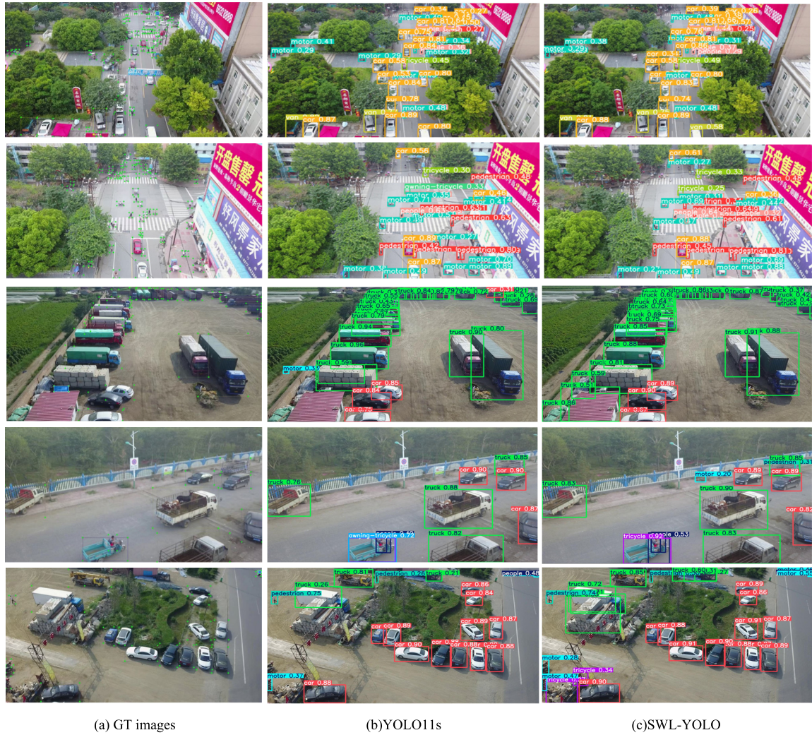
FIGURE 10. The visualization results on two datasets. While the baseline detector YOLO11s falsely detects or misses the small targets, the proposed SWL-YOLO detector can correctly detect the target objects.
