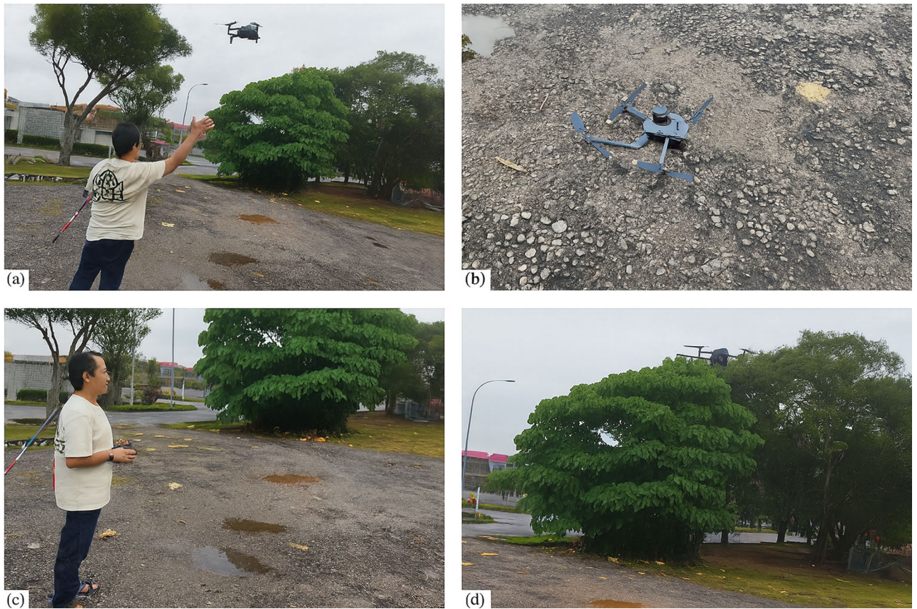
Fig. 2. Field operation of drone-based aerial survey in Sect. 24, Shah Alam. (a) UAV operator performing manual launch sequence under controlled open-site conditions; (b) DJI Phantom 4 Pro deployed on pre-flight calibration ground point; (c) aerial take-off procedure during vegetation–shade mapping missions. All operations complied with Civil Aviation Authority of Malaysia (CAAM) regulations and institutional ethical standards.
