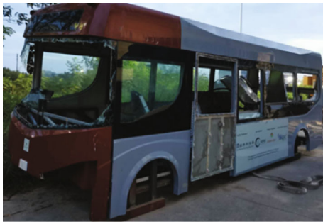
FIGURE 27: Sandwich body after FRB test.
