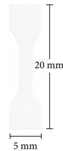
FIGURE 3: Tensile specimen of sandwich material.
