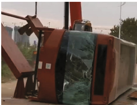
FIGURE 28: Sandwich body after R66 test.
