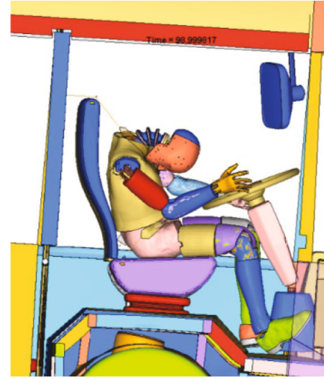
FIGURE 16: Dummy dynamics at 120 ms.
