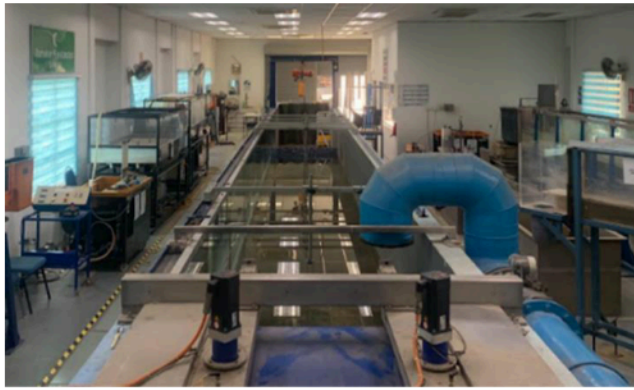
Figure 2 Wave flume in Hydraulic laboratory of Civil Engineering Department, Universiti Putra Malaysia
