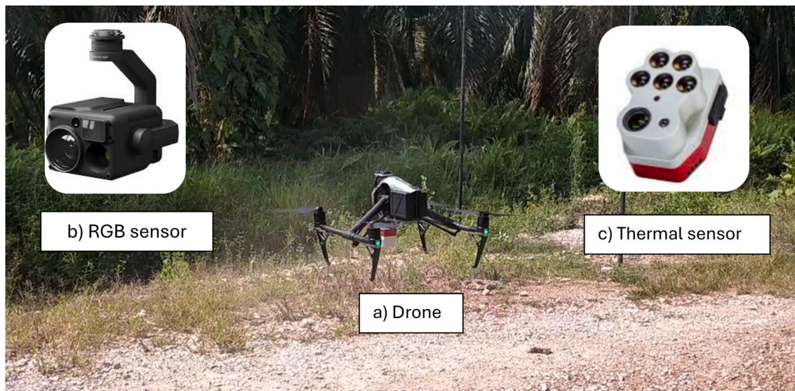
Fig. 4. a) DJI Inspire 2 drone, b) DJI Zenmuse H20 camera and c) Mica Sense Altum-PT sensor.
