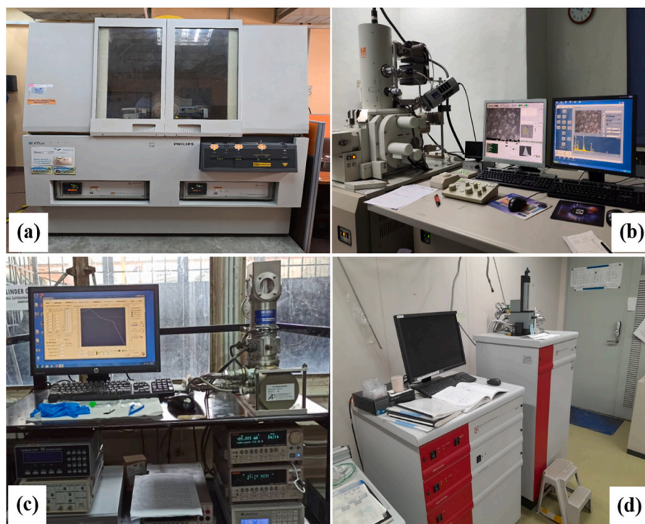
Fig. 2. Photographic representation of physical instruments used in this study: (a) X-ray diffraction (XRD); (b) FESEM-EDX system; (c) four-point probe (4 PP); (d) SQUID magnetometer.
