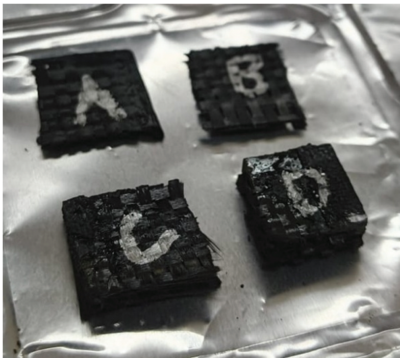
Figure 6. Burnt specimens for FESEM analysis; (a) CARALL; (b) CARALL + SiC; (c) CFFRAL; (d) CFFRAL + SiC.
