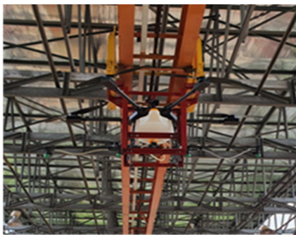
Fig. 6. The UAV was mounted on a facility at a height of 2.5 m from the ground.
