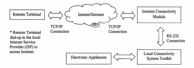
Figure 1.1: Block diagram of a complete Internet connectivity system
