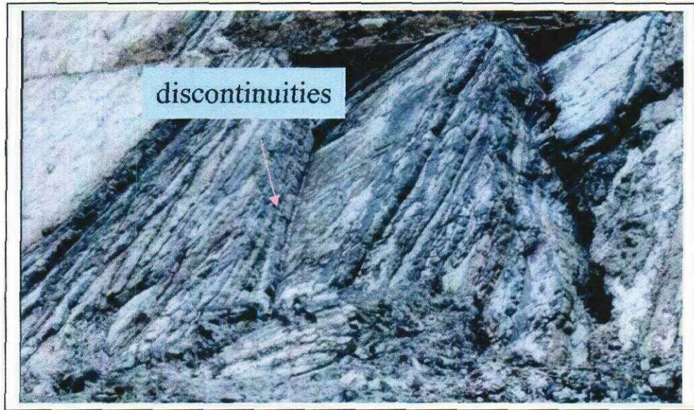
Figure 2.1: The discontinuities at CH 76000 of East Coast Expressway (2002)
