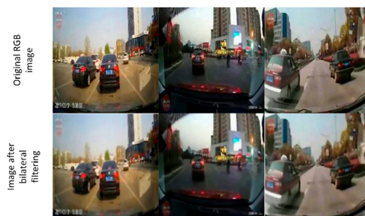
Figure 3. Bilateral filtering enhancement on RGB video frames.
