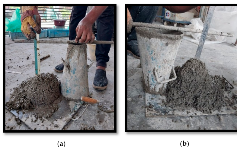
Figure 11. GPC slump at (a) 0% and (b) 20% CR replacement.
