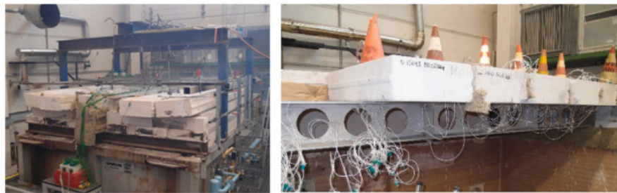
FIGURE 1. Experimental procedure perforated CSSBs expose to fire (Cashell et al. 2021)
