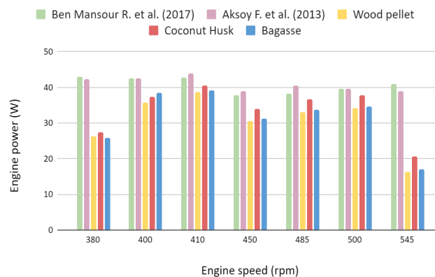
Fig. 8 Comparison between engine power with biomass waste as heat source with previous studies by Aksoy and Cinar (2013) and Ben-Mansour et al. (2017).
