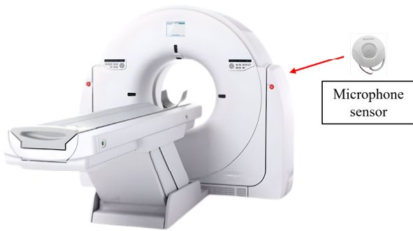
FIGURE 5. Setup of the microphone sensor on the CT scan machine.
