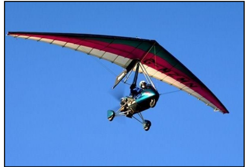
Fig. 12. Microlight flying with membrane 3-dimension airfoil
