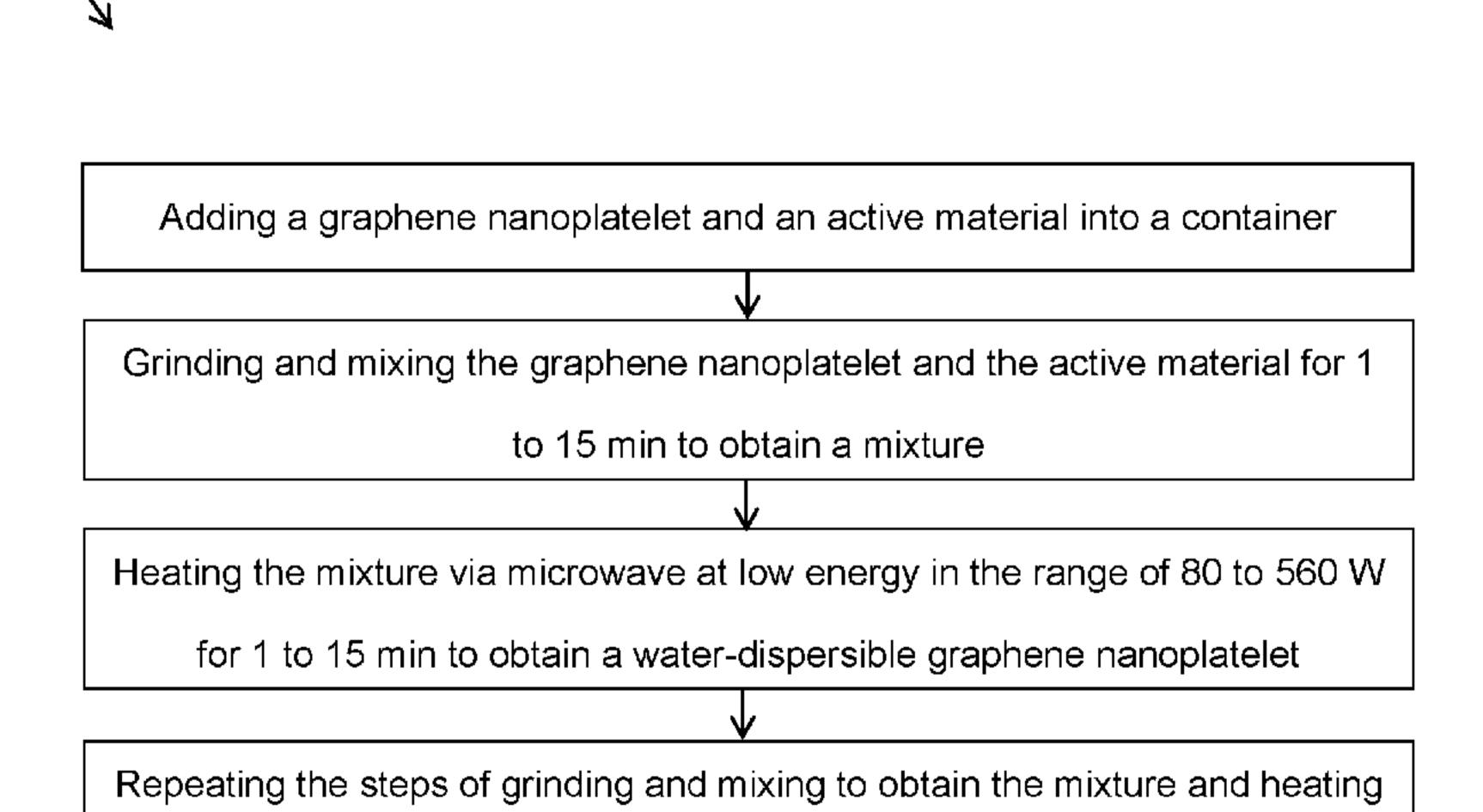
the mixture as desired to obtain the water-dispersible graphene nanoplatelet
