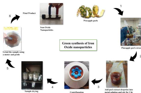
Fig. 2. Steps of green synthesis of MNPs
