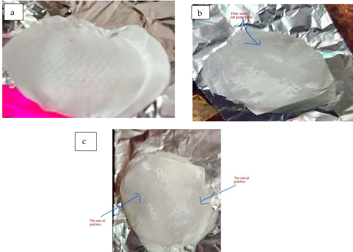
Figure 5: (a) shows the oil droplets on the membrane from SOW 1 and (b&c) represent oil patches on the membrane from SOW 2, both membranes are before the drying process
