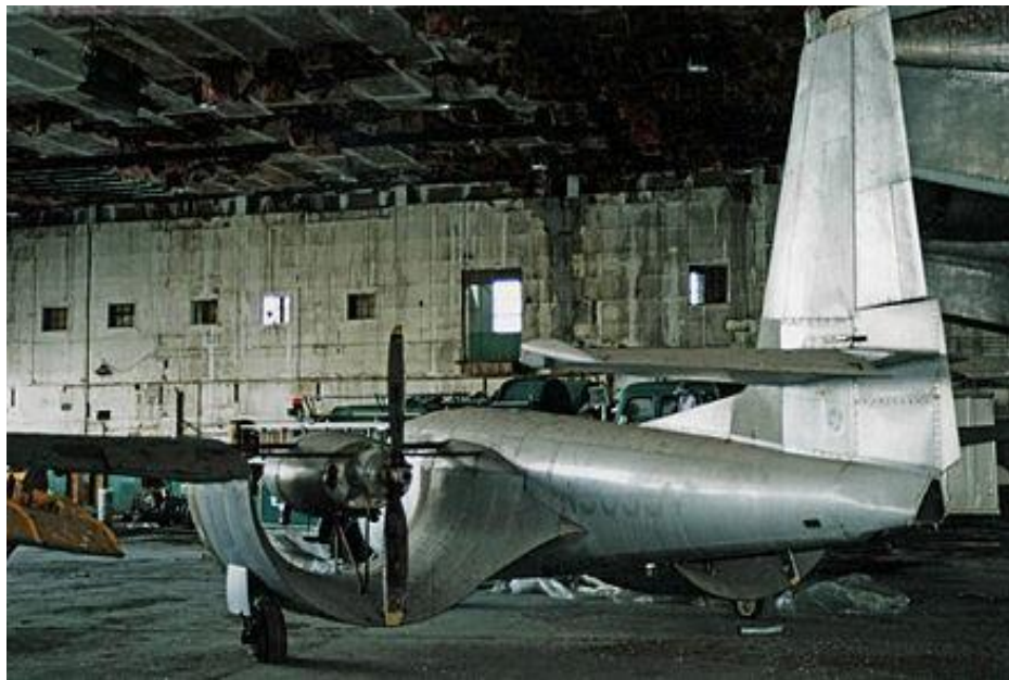
Figure 5: The propeller location for CCW-5 aircraft [24]
