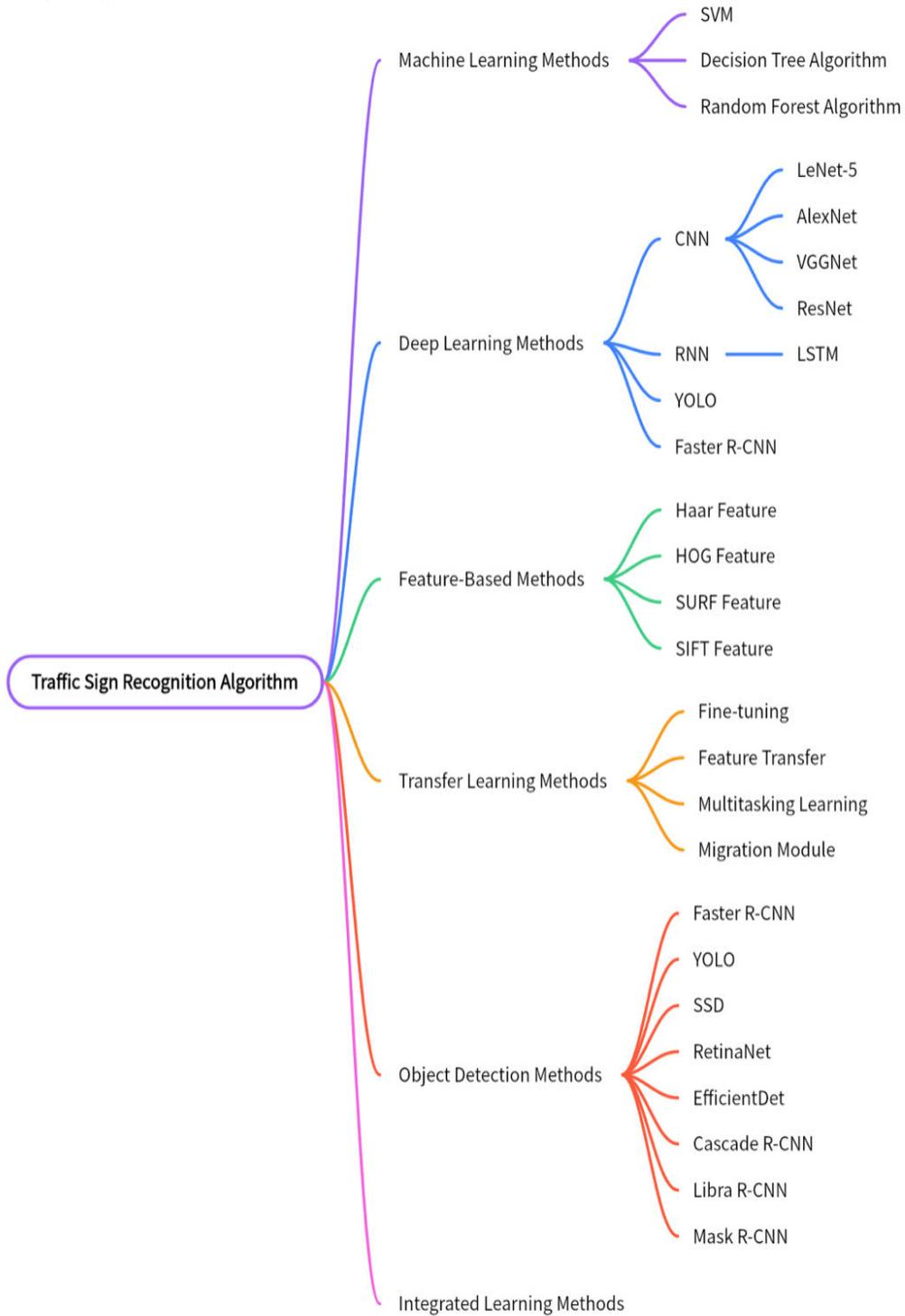
Figure 2: The classification of traffic sign recognition algorithms.
