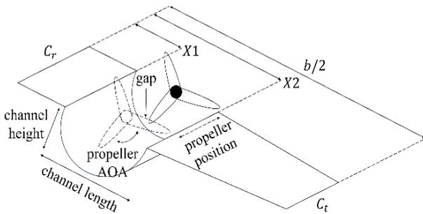
Figure 7 Channel wing geometric parameters
