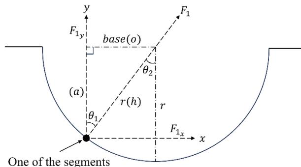
Figure 4 Free body diagram on the channel
