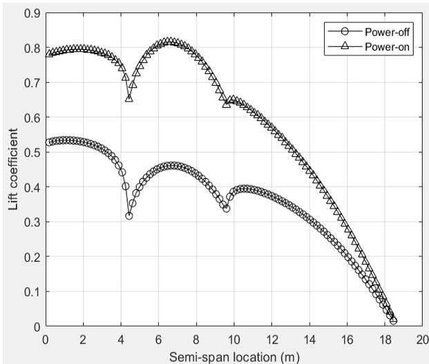
Figure 8 Channel wing lift distribution
