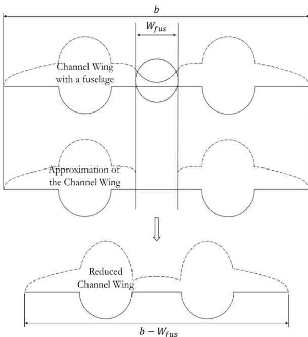
Figure 5 Accounting for a fuselage in the lifting line method
