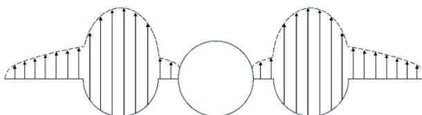
Figure 3 Expected lift distribution of the power-on channel wing
