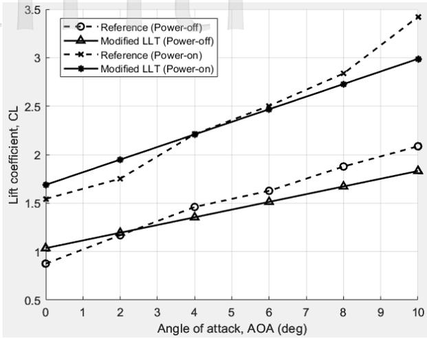
Figure 6 Comparison of the reference model and modified lifting line method
