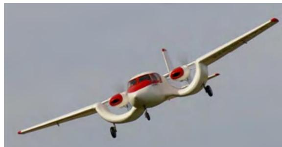
Figure 1 Example of channel wing aircraft design [4]
