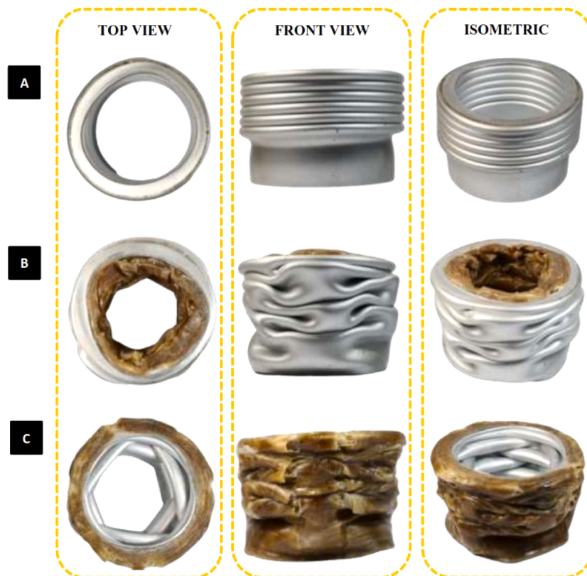
Fig. 10. Final deformation under quasi-static loading (a) ACT (b) HICT (c) HOCT.
