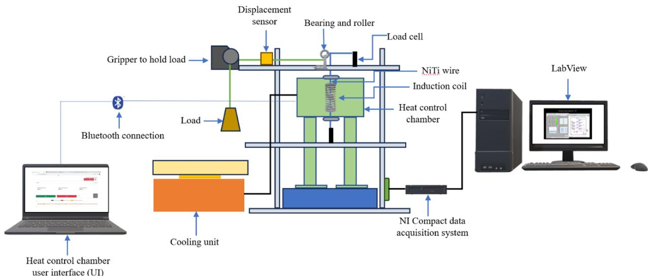
Figure 2 Experimental set-up for loading configuration with induction heating
