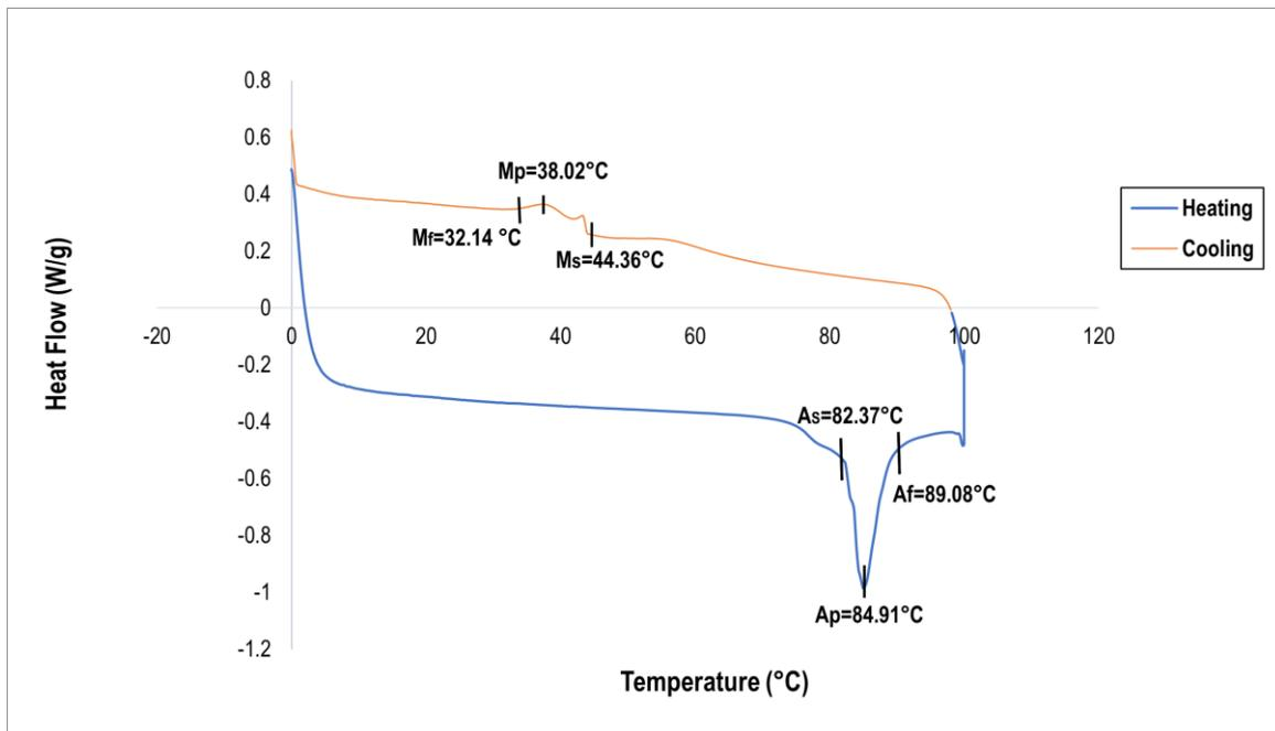
Figure 4 DSC results for NiTi Flexinol Wire
