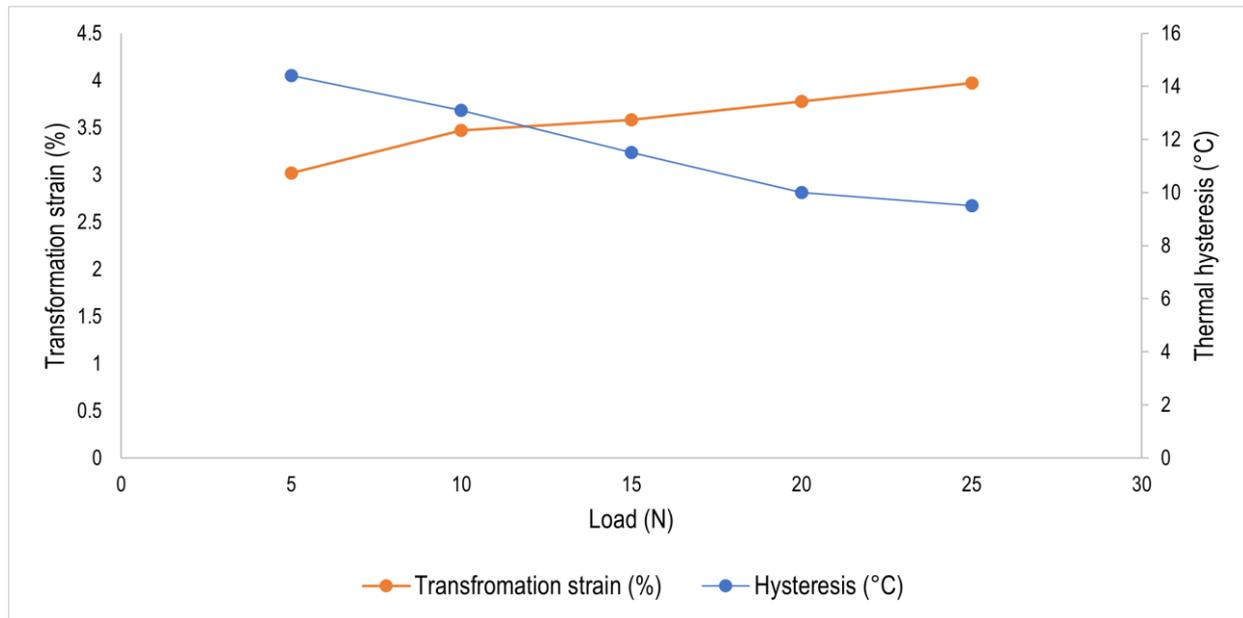
Figure 8 Relationship between Thermal Hysteresis and Transformation Strain
