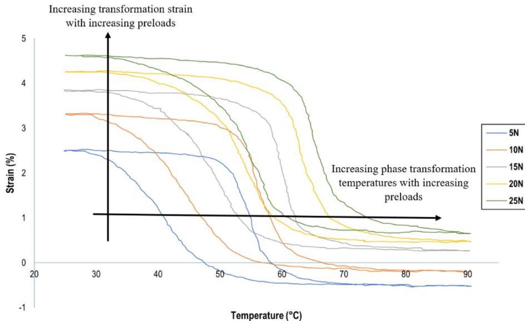
Figure 5 SME Behaviour of NiTi Flexinol Wire at Different Preloads
