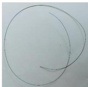
(b) Experimental sample of Flexinol actuator wire
