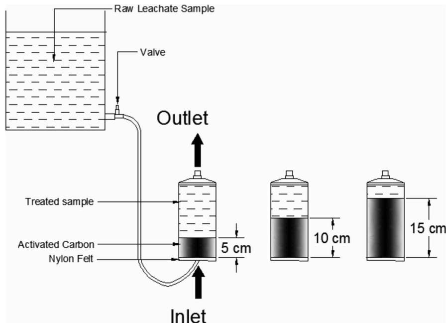
**Fig. 3.** Up flow AC contactor.
