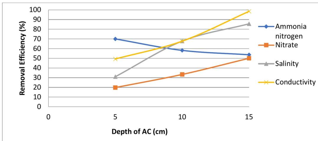
**Fig. 8.** Removal efficiency of ammonia nitrogen, nitrate, salinity and electrical conductivity by activated carbon adsorption.
