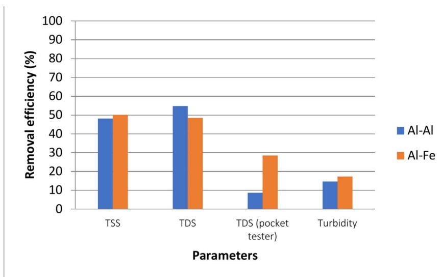
**Fig. 4.** Removal efficiency of TSS, TDS and turbidity by electrolysis.
