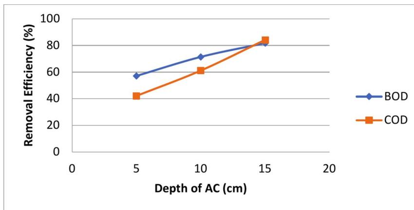
Fig. 6. Removal efficiency of BOD and COD by activated carbon adsorption.
