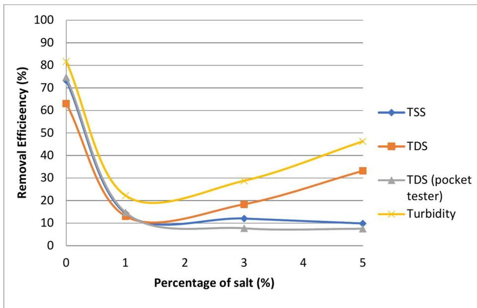
**Fig. 10.** Removal efficiency of TSS, TDS and turbidity by electrolysis and activated carbon adsorption.
