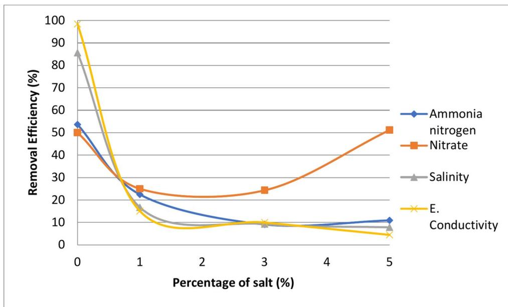
**Fig. 11.** Removal efficiency of ammonia nitrogen, nitrate, electrical conductivity and salinity by electrolysis and activated carbon adsorption.
