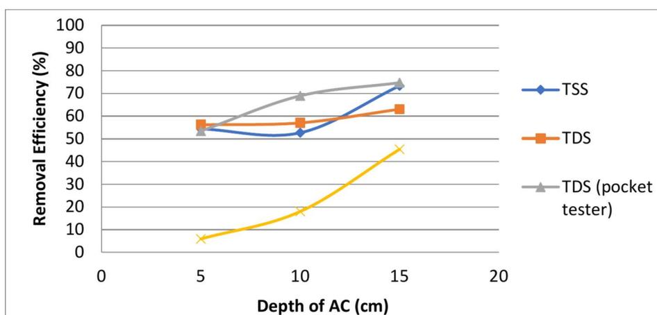
Fig. 7. Removal efficiency of TSS, TDS and turbidity by activated carbon adsorption.
