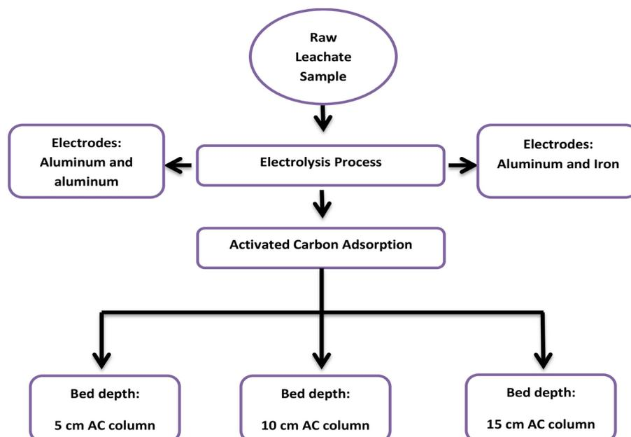
Fig. 1. Flow chart of the treatment process.
