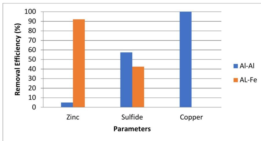
**Fig. 5.** Removal efficiency of zinc, sulfide and copper by electrolysis.
