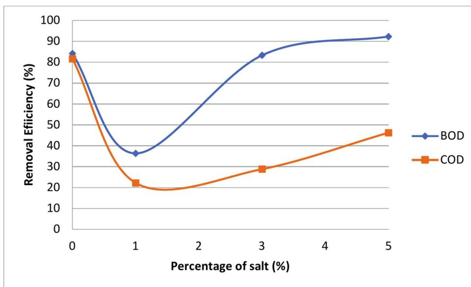
**Fig. 9.** Removal efficiency of BOD and COD by electrolysis and activated carbon adsorption.
