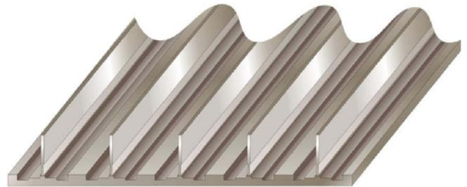
Fig. 9. Schematic representation of a crenellated test panel [72].
