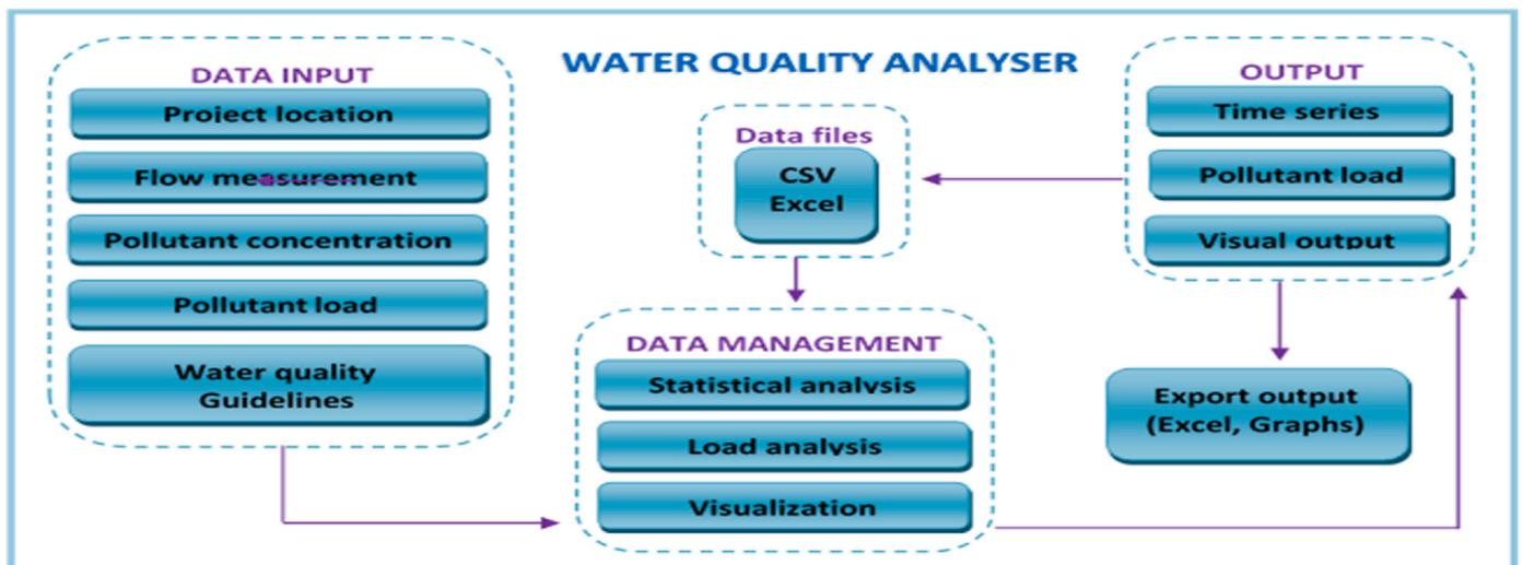
Fig. 2. Simplified architectural design of the Water Quality Analyser (WQA).
