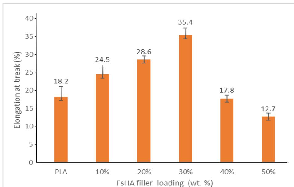
**Figure 6:** Elongation at break of PLA/FsHA composite with various amount of FsHA filler loading
