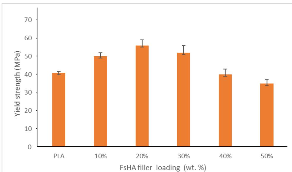
**Figure 5:** Yield strength of PLA/FsHA with various composites of filler loading
