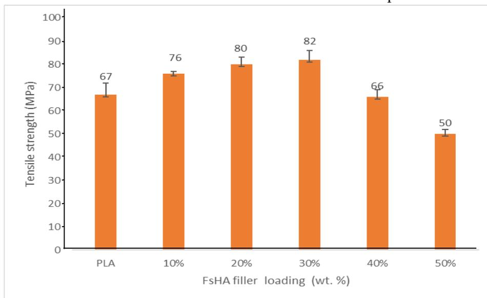
**Figure 4:** Tensile strength of PLA/FsHA with various amount of filler loading
