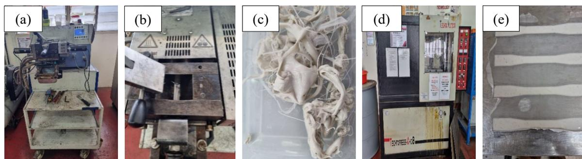
**Figure 1:** Process of producing PLA/FsHA by using internal mixer (Brabender), (a) Internal mixer (Brabender), (b) top view from the internal mixer on blending the sample, (c) sample produced from internal mixer, (d) hot and cold press (Technovation) (e) tensile specimen of the composites from the mould
