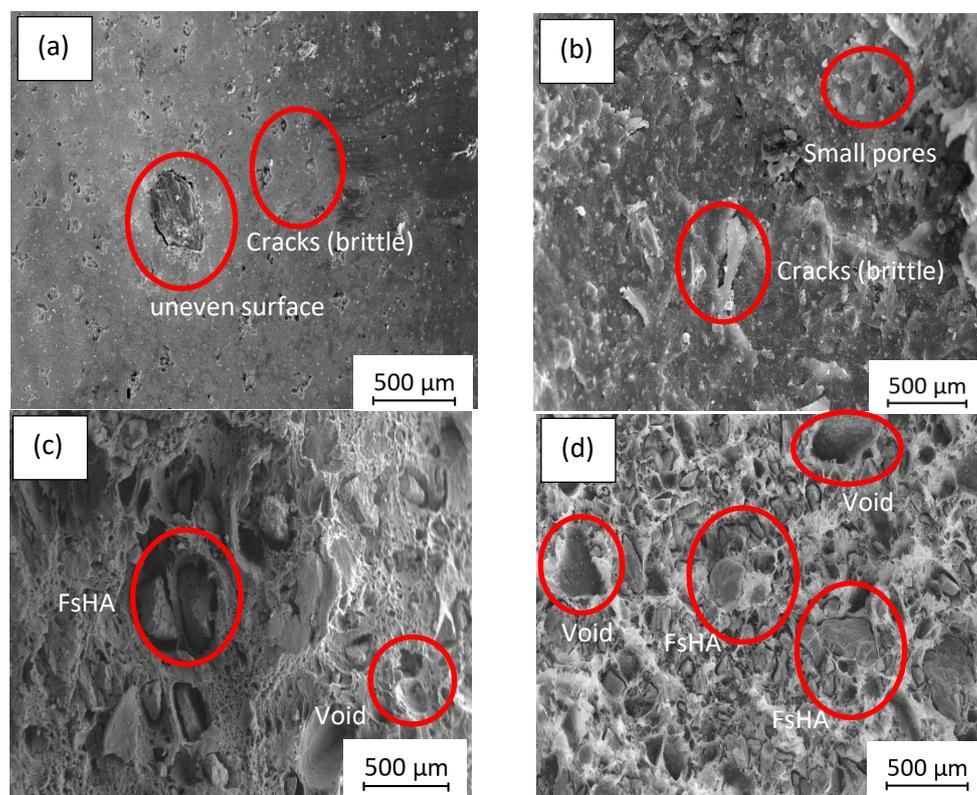
**Figure 7:** FESEM micrographs of fracture surface (a) pure PLA, (b) PLA/10FsHA, (c) PLA/30FsHA, and (d) PLA/50FsHA
