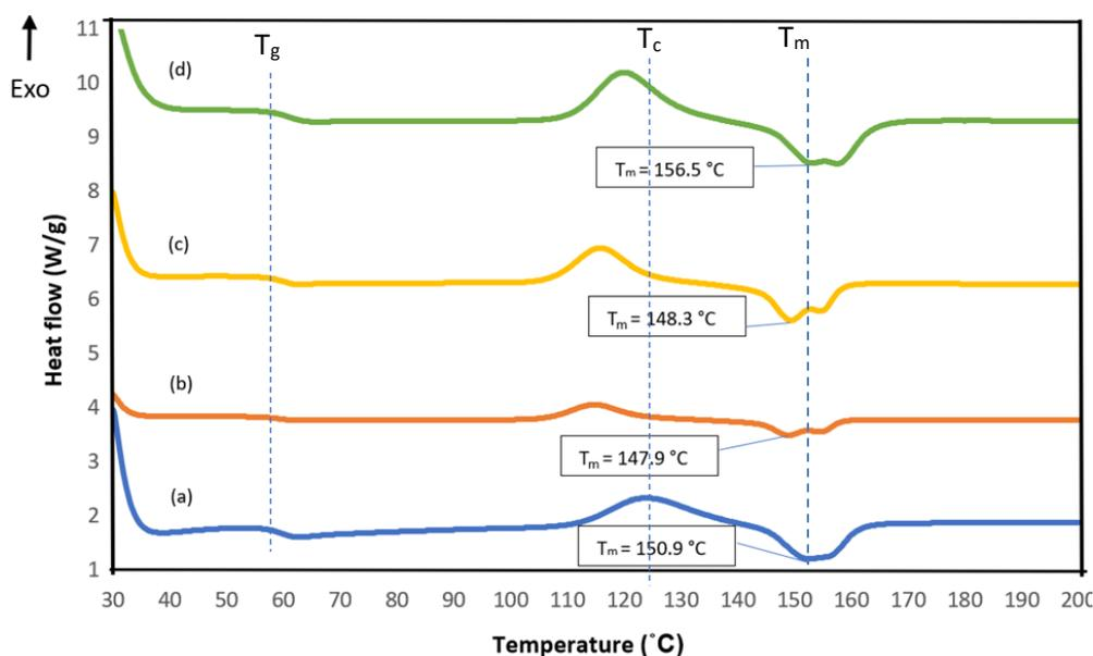
**Figure 3:** DSC melting thermograms of (a) pure PLA, (b) PLA/10FsHA, (c) PLA/30FsHA and (d) PLA/50FsHA
