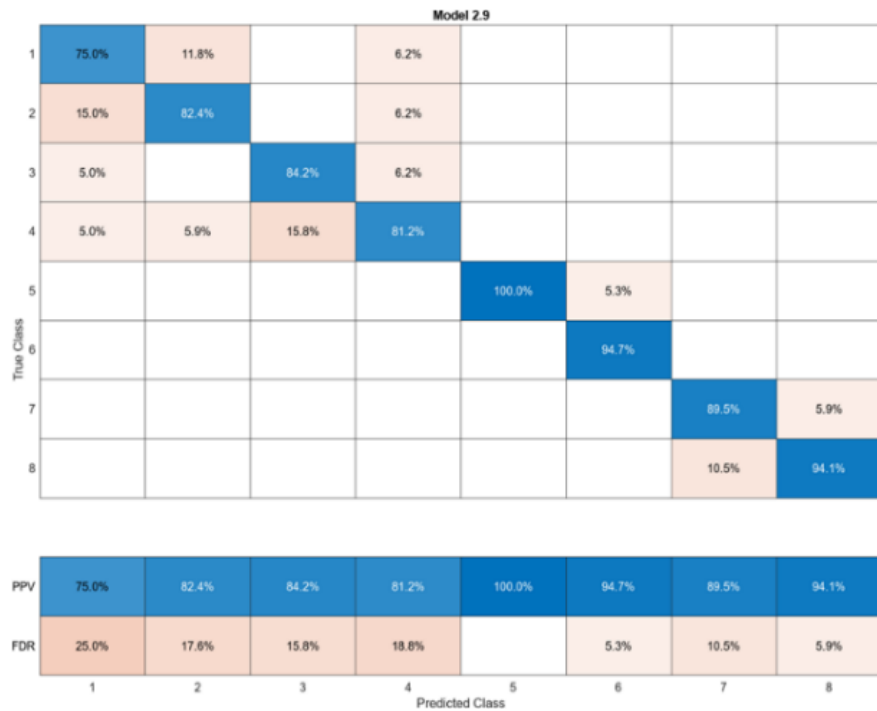
Figure 11 QSVM Confusion Matrix for acceleration data
