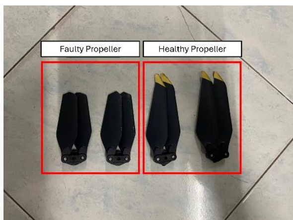
Figure 5 Healthy and faulty propeller. The faulty propeller's tip is cut by 15mm to simulate faults
